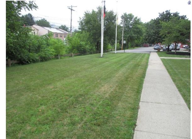
Two rain gardens can be set up in the turfgrass areas adjacent to the building to capture stormwater from the rooftops of the buildings. A preliminary soil assessment suggests that the soils have suitable drainage characteristics for green infrastructure.
