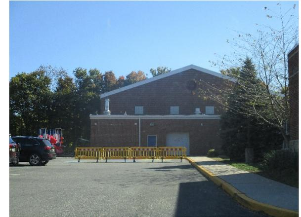
Porous pavement can be installed on the northern and eastern parking strips to capture stormwater from the parking lot. Downspout planter boxes can be constructed along the northeastern edge of the building to allow roof runoff to be reused. A preliminary soil assessment suggests that more soil testing would be required before determining the soil's suitability for green infrastructure.
